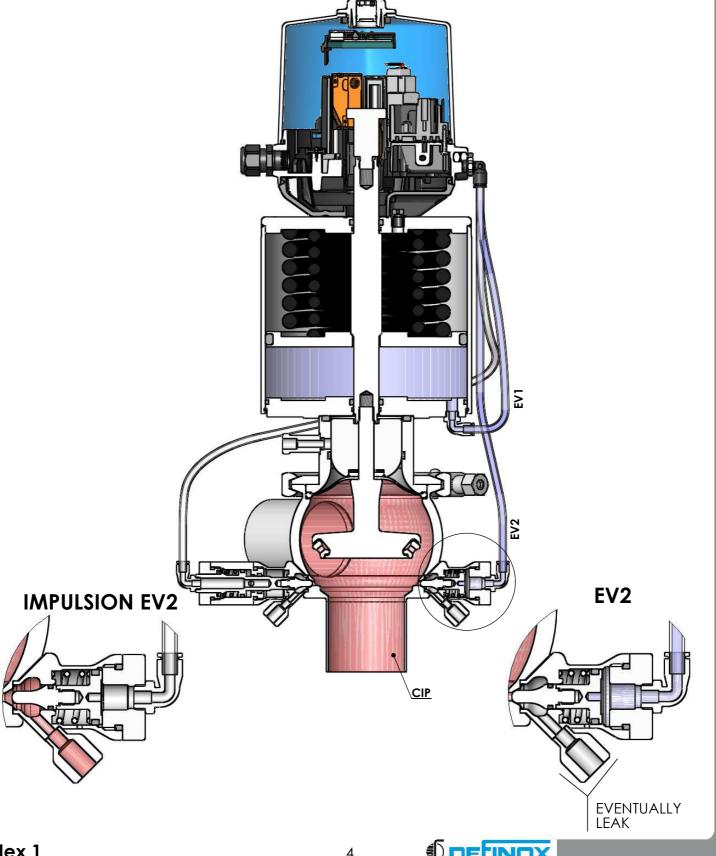
1 LEAKAGE VALVE - with control 1 CLEANING VALVE - with control 3 SOLENOÏD VALVE (3 SV)
