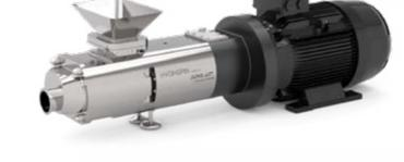
The HYGHSPIN Hopper is an extension to the worldwide proven HYGHSPIN stainless steel pump series. This innovative twin screw pump is able to transport easily products with high viscosities. The feed screws are extended so that they can draw in non-flow capable products below the inlet and feed them into the pump chamber. This ensures particularly gentle handling – no need for external feeding equipment.
